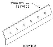
bare metal thickness (t) = 0.0538 in. (1.37mm)
